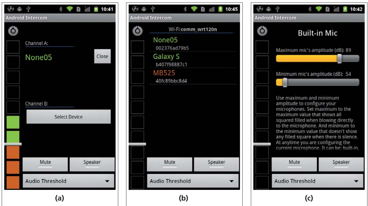
■ Figure 6. Android Intercom application: Bluetooth mode screen (a), Wi-Fi mode screen (b) and microphone preferences screen (c).
